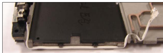
< 4. ANTENNA CONNECTOR WIRE 안착 >
