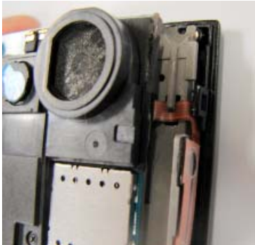
notice interference between VOLUME KEY FPCB and FRONT RIB
