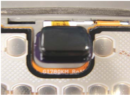
inset the OPTICAL MOUSE FPCB into the BRACKET hole
