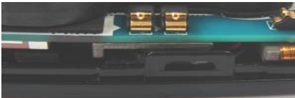
notice interference between VOLUME KEY FPCB and FRONT RIB
