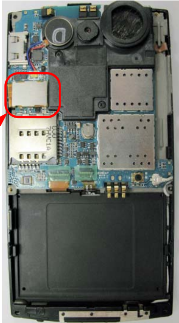
notice interference between VOLUME KEY FPCB and FRONT RIB
