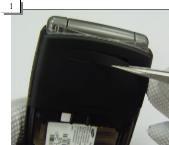
Remove the Rear Screw Deco
