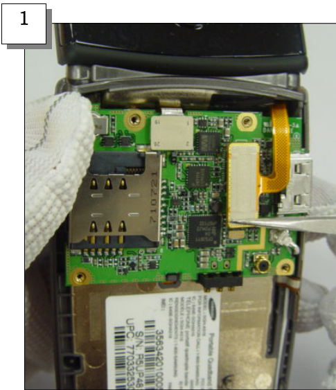
Disjoint the LCD Connector
