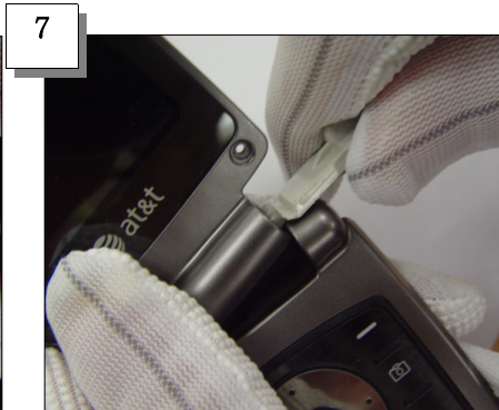
Join the Lower to the Front by using the lever like the picture 6, 7 and 8
