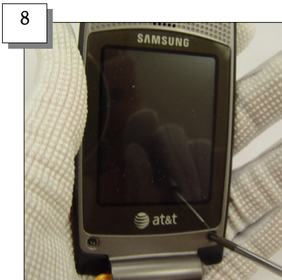
8 Tighten the Screws (2 Points)
