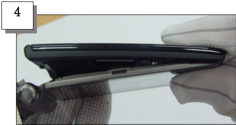
4 Join the Upper to the bottom of the Lower
