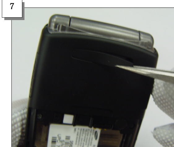
Attach the Rear Screw Deco
