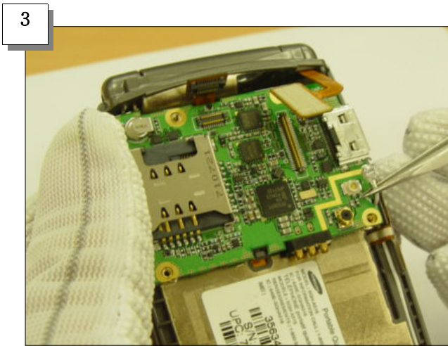
Join the PBA to the Front (Put the Antenna wire in the hole in the PBA)
