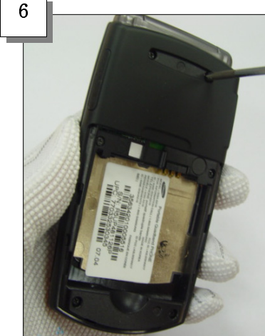
Tighten the Screws (6 Points)
