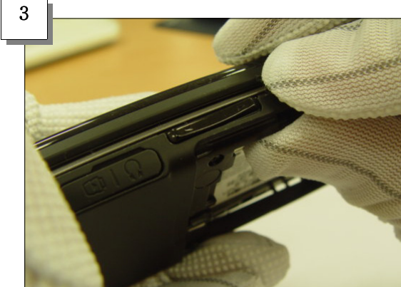
Join the Sidekey between Front and Rear
