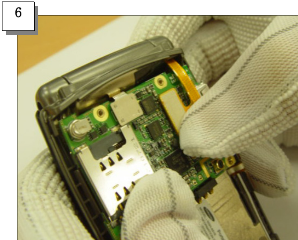
Assemble the LCD Connector
